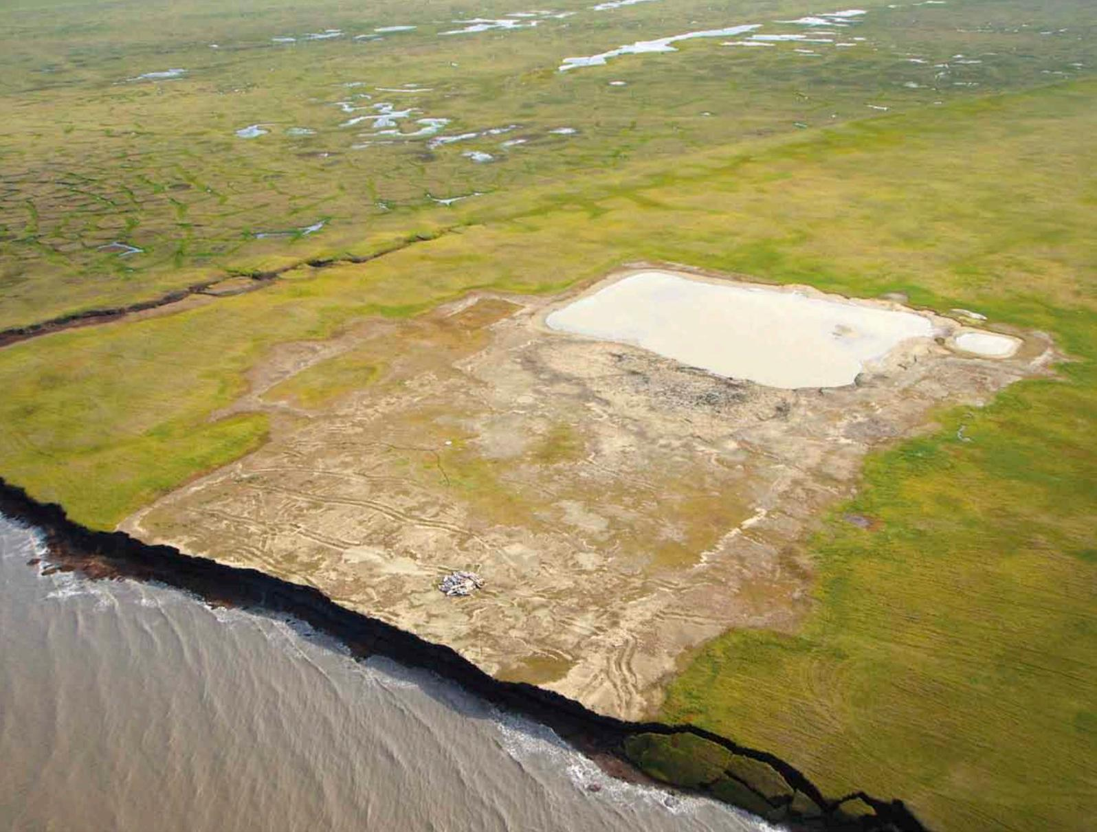
This petroleum test well drilled near Drew Point in the winter of 1977–78 had to be capped in 2010 by the Bureau of Land Management because the coast was rapidly approaching the original structures, some of which can still be seen on the drill pad after mitigation was completed.
