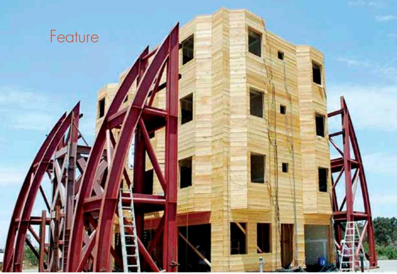
A soft-story wood-frame apartment building under construction in 2013 on the shake table at the University of California at San Diego (UCSD).
