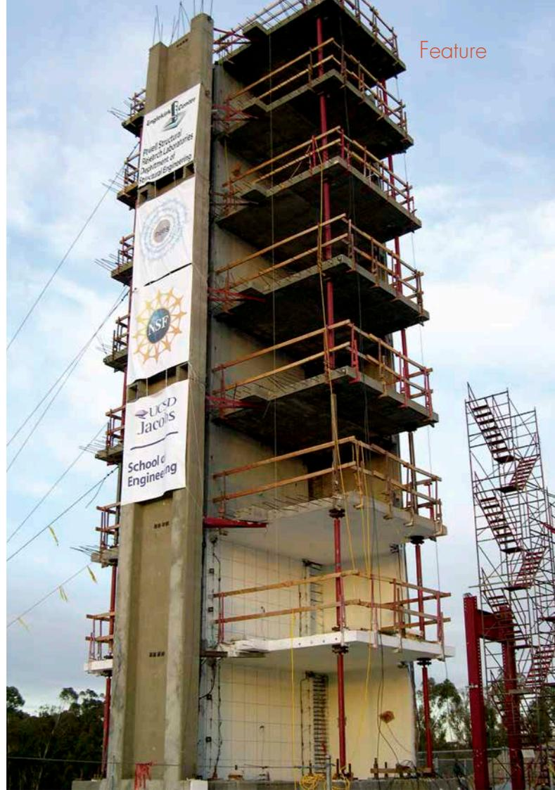
A slice of a seven-story reinforced concrete building ready for testing on the UCSD shake table facility.
